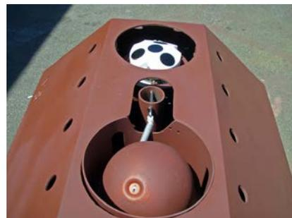
**Figure 9.** Trawl Resistant Bottom Mount with Acoustic Release
