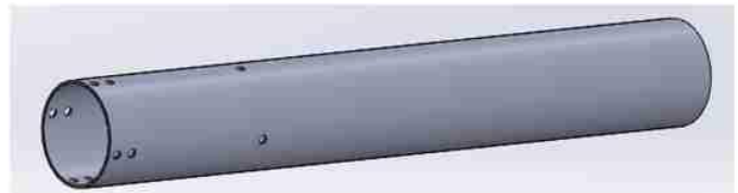
Fig. 6. Outer pipe for engine and shaft adapter
