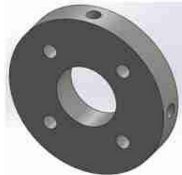
Fig. 5. Connection piece shaft adapter – engine
